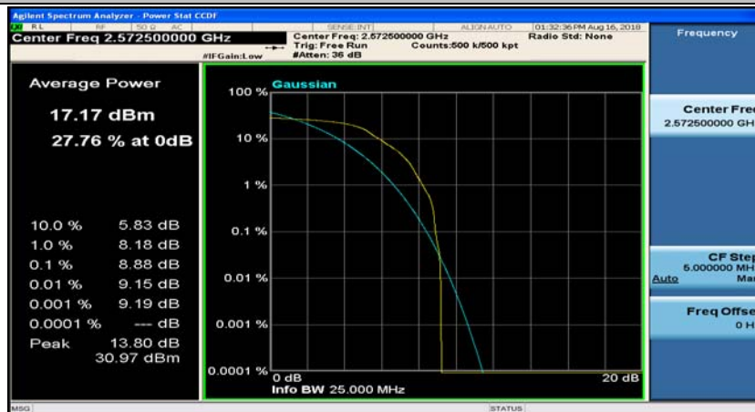
(Channel Bandwidth: 5 MHz)_LCH_QPSK_1RB#24
