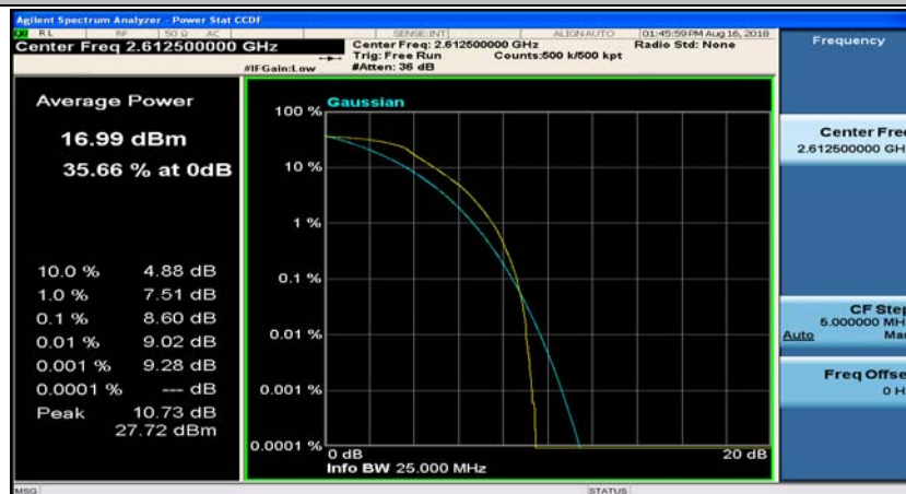
(Channel Bandwidth:15 MHz)_HCH_QPSK_75RB#0
