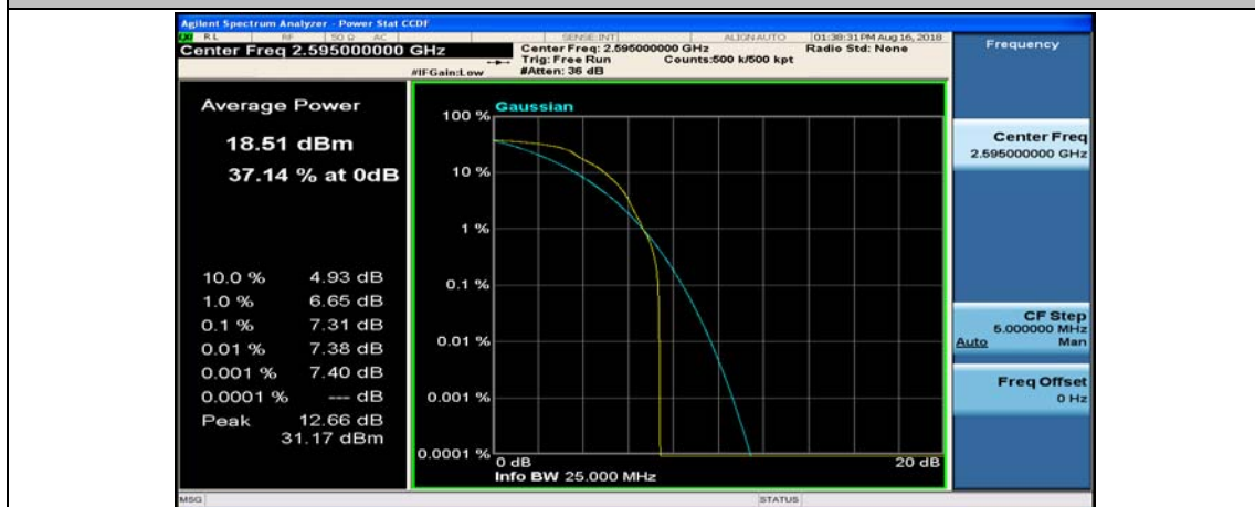
Channel Bandwidth: 10 MHz_MCH_QPSK_1RB#49
