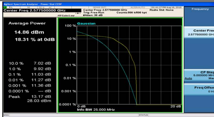
(Channel Bandwidth:15 MHz)_LCH_QPSK_1RB#37
