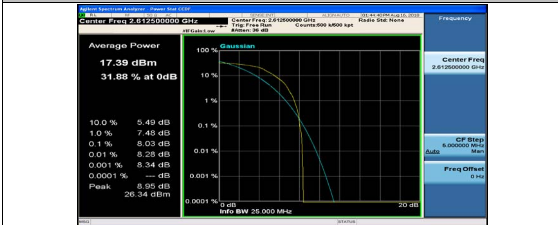
(Channel Bandwidth:15 MHz)_HCH_QPSK_1RB#37
