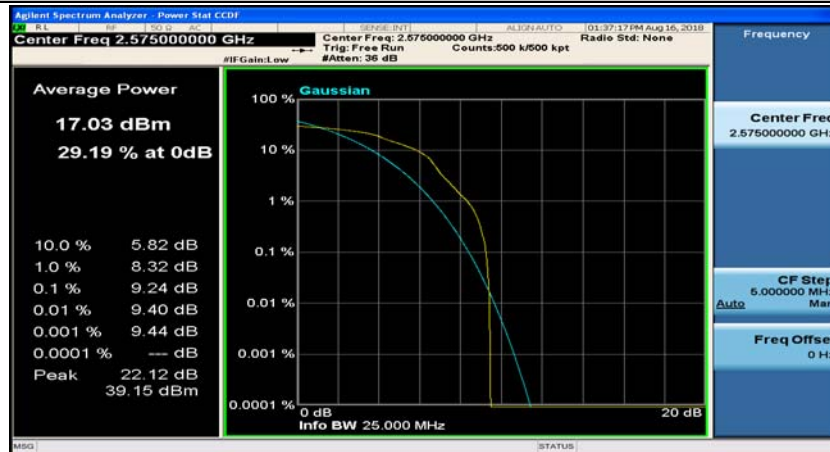
Channel Bandwidth: 10 MHz_LCH_16QAM_1RB#49
