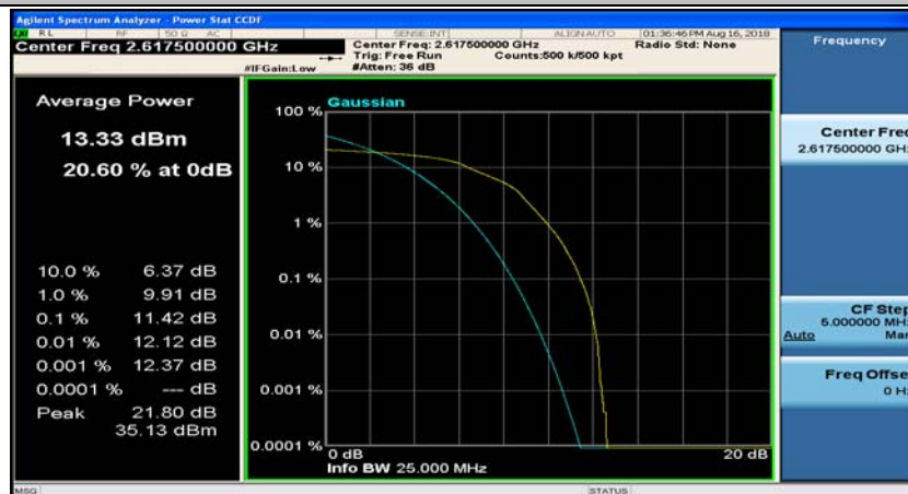
(Channel Bandwidth: 5 MHz)_HCH_16QAM_25RB#0
