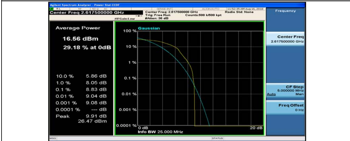
(Channel Bandwidth: 5 MHz)_HCH_16QAM_1RB#12
