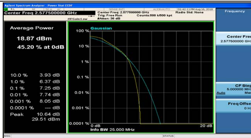
(Channel Bandwidth:15 MHz)_LCH_QPSK_37RB#38
