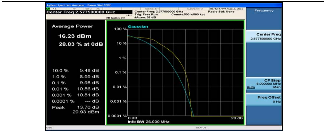
(Channel Bandwidth:15 MHz)_MCH_QPSK_1RB#0
