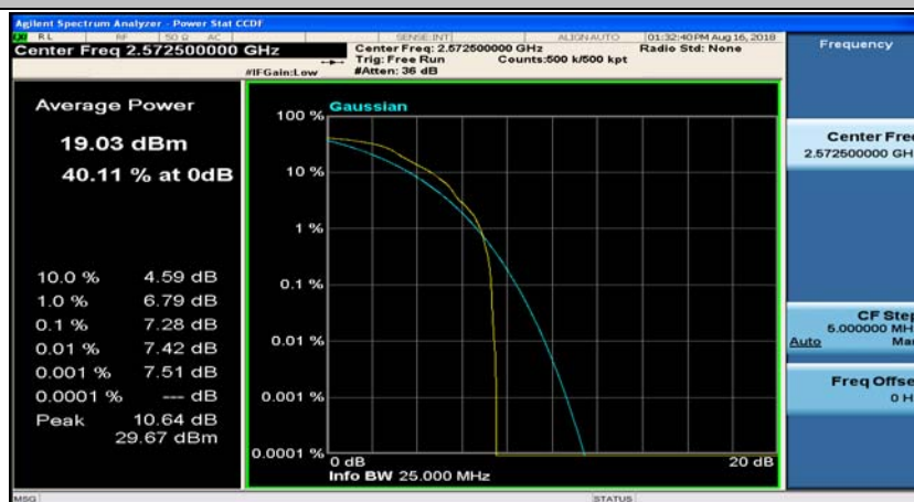
(Channel Bandwidth: 5 MHz)_LCH_QPSK_12RB#0
