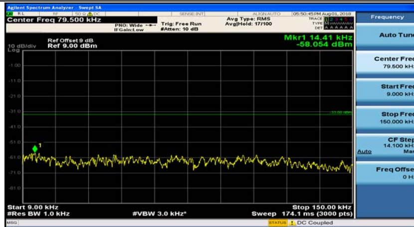
(Channel Bandwidth: 5 MHz)_LCH_16QAM_1RB#0
