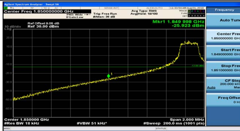
(Channel Bandwidth:15 MHz)_LCH_16QAM_1RB#37
