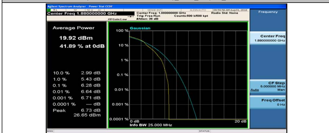
(Channel Bandwidth: 5 MHz)_MCH_16QAM_1RB#12
