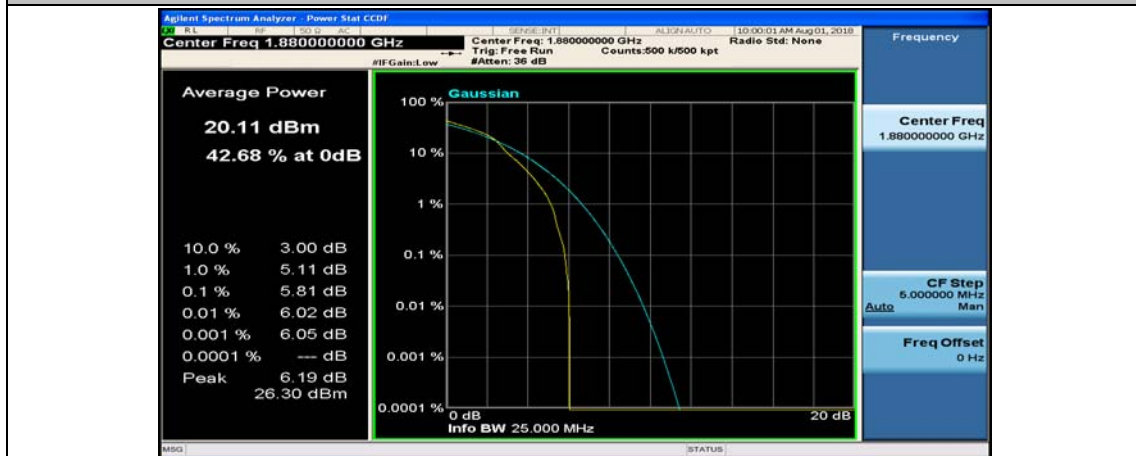
(Channel Bandwidth: 5 MHz)_MCH_16QAM_1RB#24
