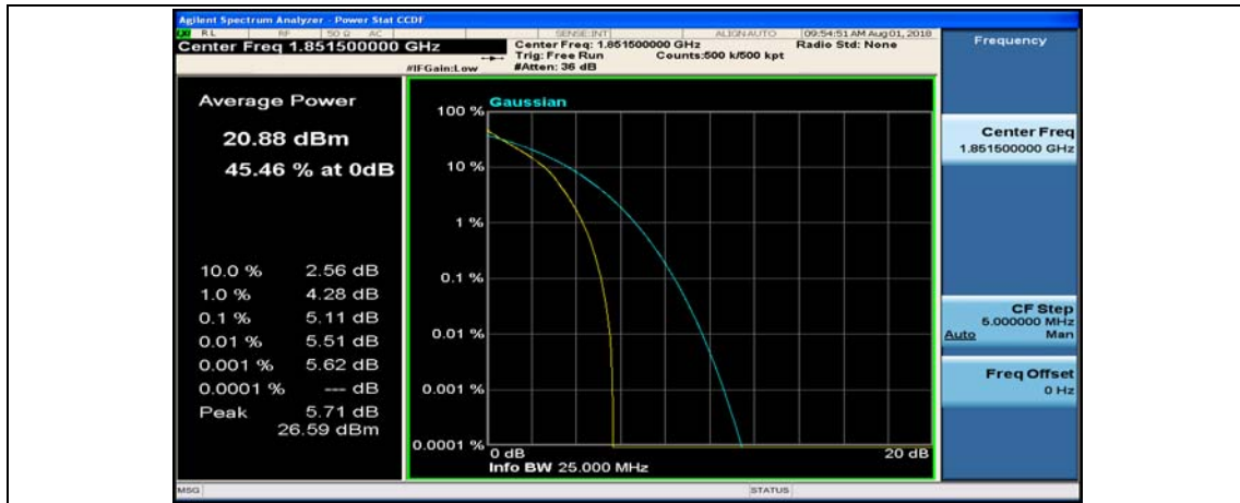
(Channel Bandwidth: 3 MHz)_MCH_QPSK_1RB#0
