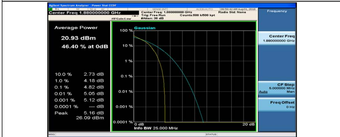
(Channel Bandwidth: 5 MHz)_MCH_QPSK_1RB#24
