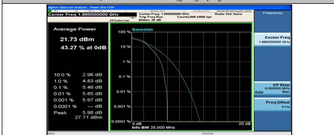
(Channel Bandwidth: 1.4 MHz)_MCH_16QAM_1RB#3
