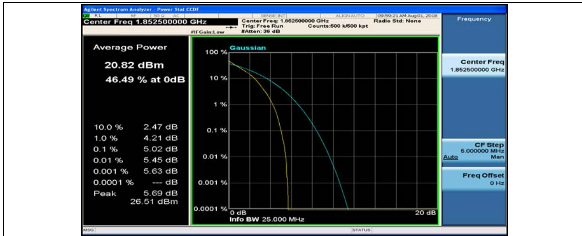
(Channel Bandwidth: 5 MHz)_MCH_QPSK_1RB#0
