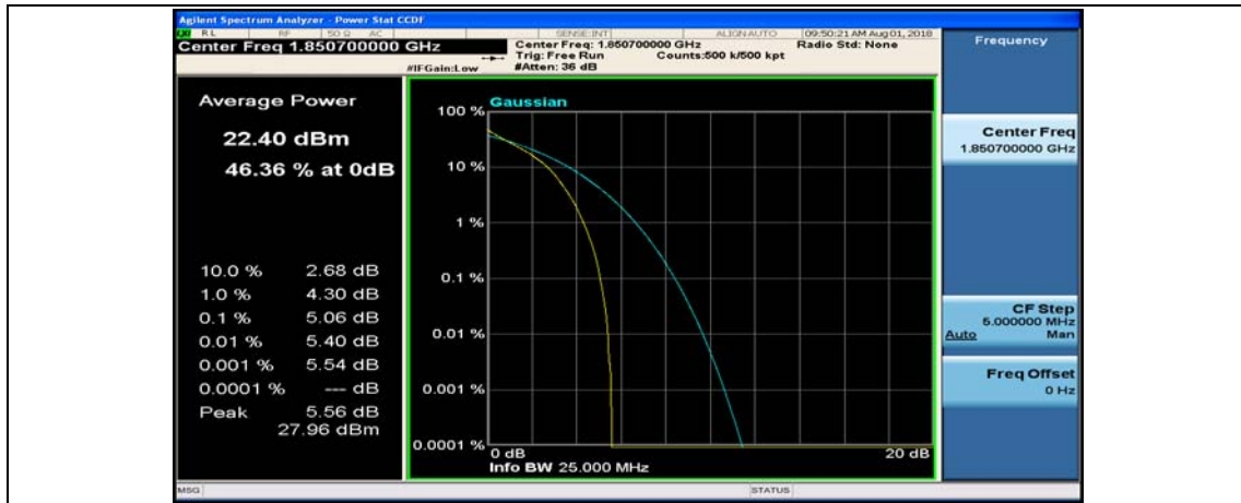
(Channel Bandwidth: 1.4 MHz)_MCH_QPSK_1RB#0
