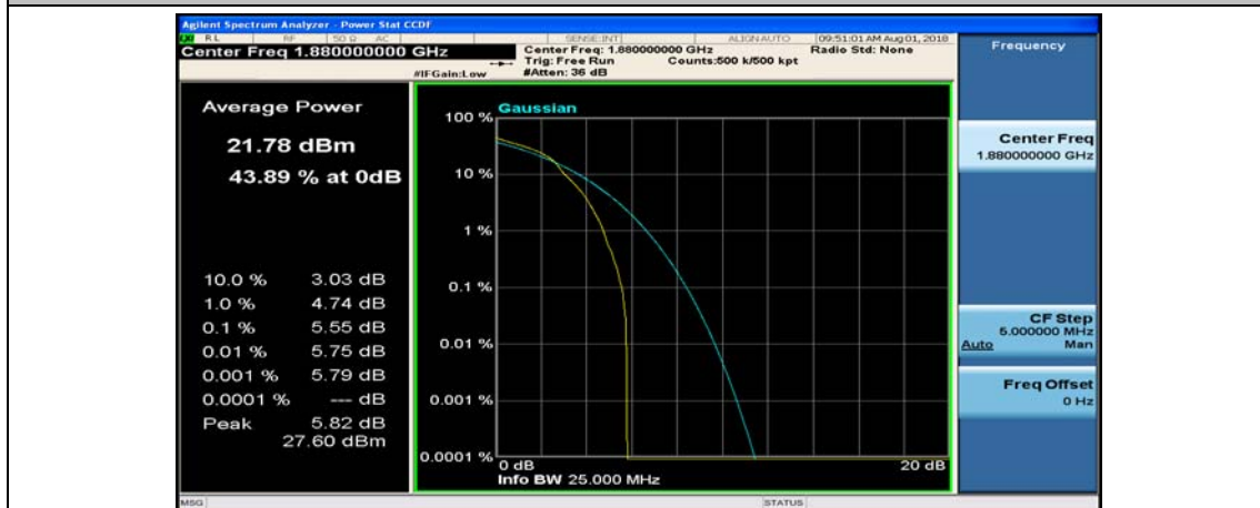
(Channel Bandwidth: 1.4 MHz)_MCH_16QAM_1RB#5
