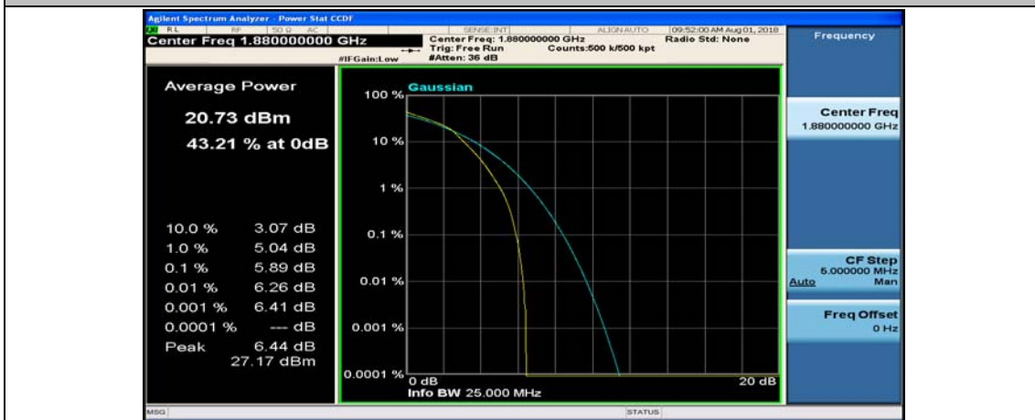
(Channel Bandwidth: 1.4 MHz)_MCH_16QAM_6RB#0
