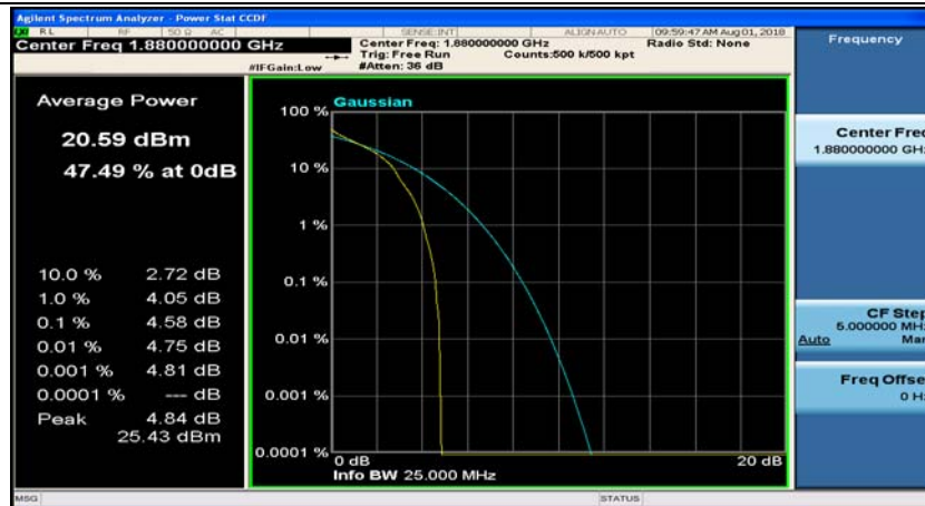
(Channel Bandwidth: 5 MHz)_MCH_QPSK_12RB#0
