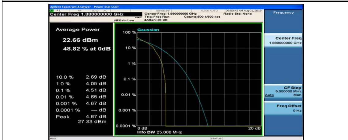
(Channel Bandwidth: 1.4 MHz)_MCH_QPSK_1RB#5
