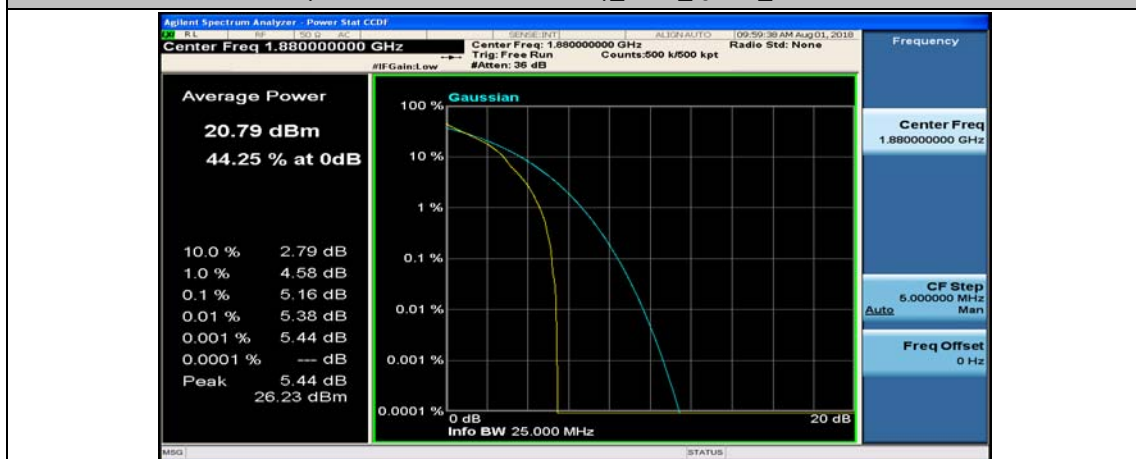
(Channel Bandwidth: 5 MHz)_MCH_QPSK_1RB#12
