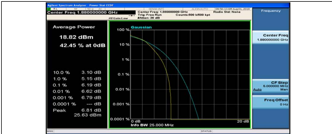
(Channel Bandwidth: 3 MHz)_MCH_16QAM_15RB#0
