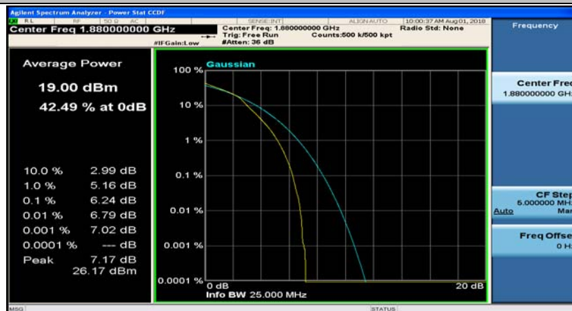
(Channel Bandwidth: 5 MHz)_MCH_16QAM_12RB#13
