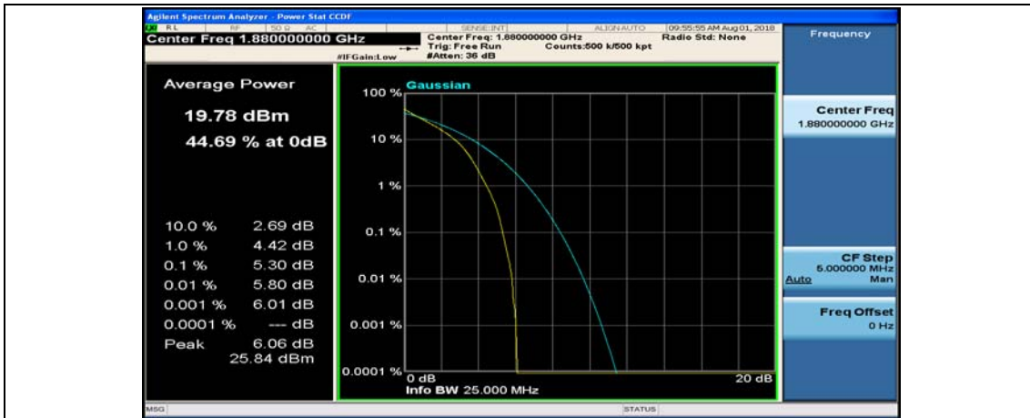
(Channel Bandwidth: 3 MHz)_MCH_QPSK_15RB#0
