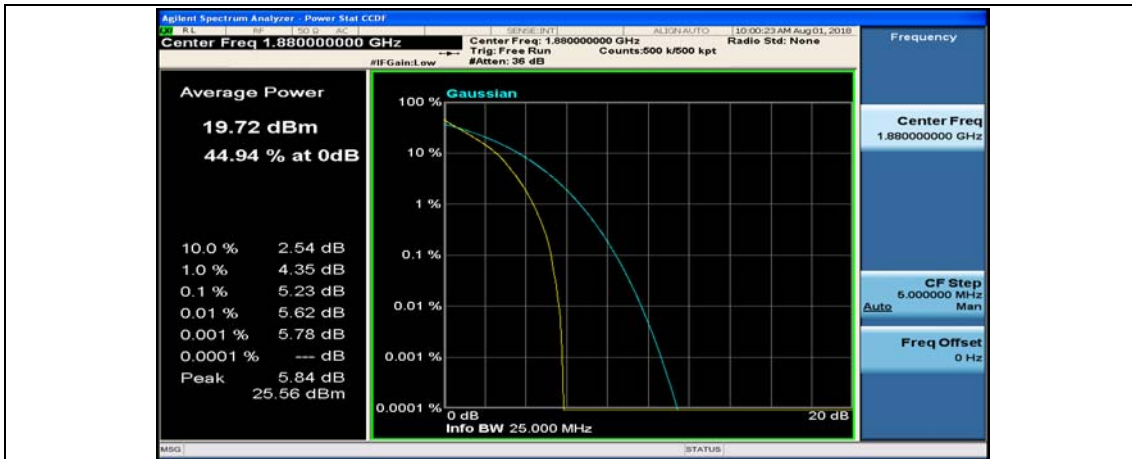
(Channel Bandwidth: 5 MHz)_MCH_QPSK_25RB#0
