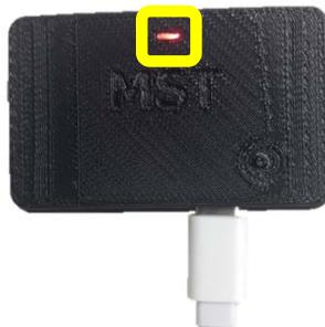
Connect the charging cable to charge as shown above
