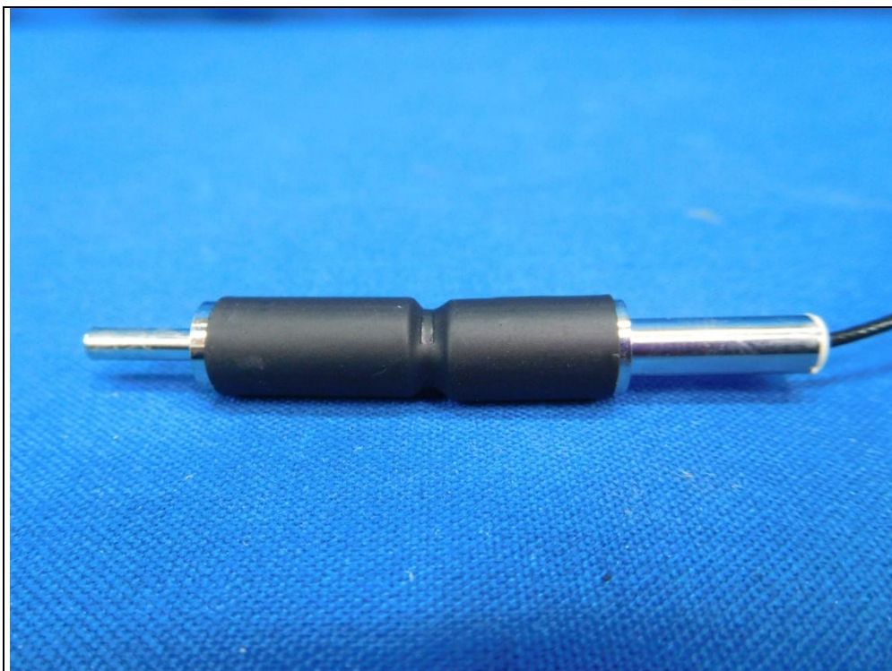
WLAN antenna No. 2
