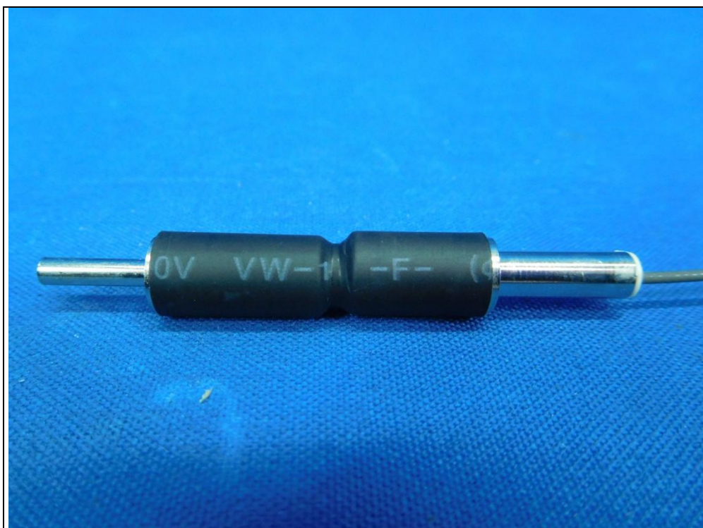
WLAN antenna No. 1
