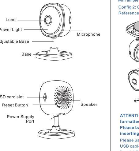
Lens, Power Light, Adjustable Base, Base, SD card slot, Reset Button, Power Supply Port, Speaker
