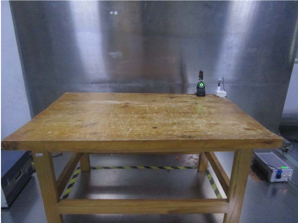
Conducted Emissions – Front View
