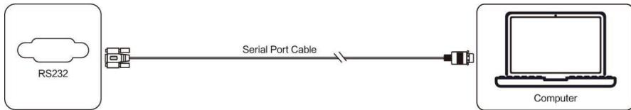
After using serial port cable to connect central control equipment and machine, certain function of the machine can be controlled via central control equipment, such as: machine ON/OFF, and adjustment of sound volume, etc.
