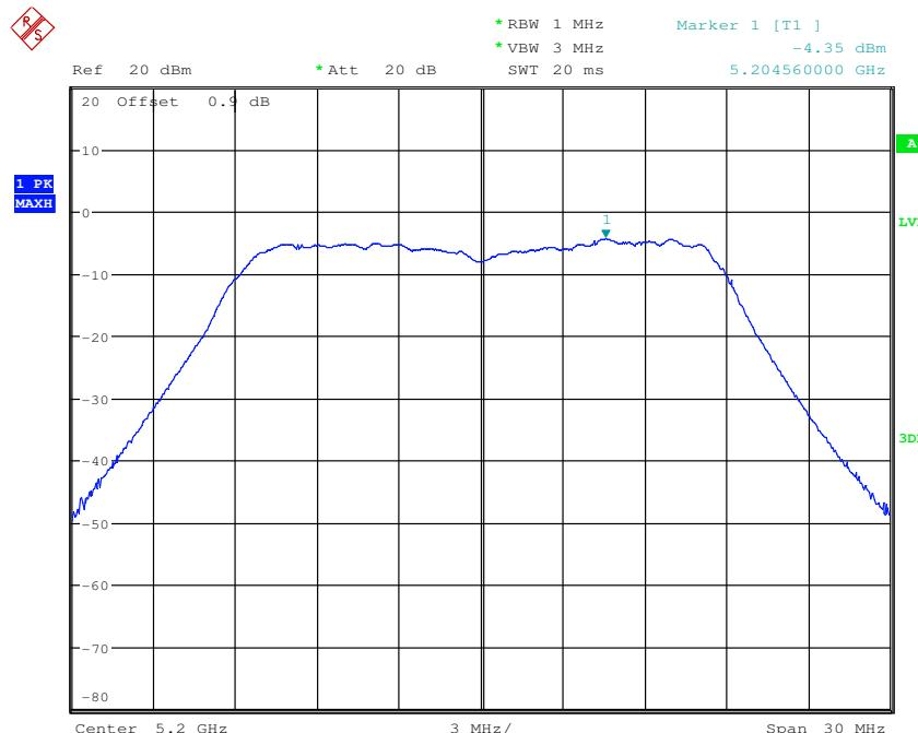
Test mode: 802.11n(HT20) Frequency(MHz): 5260
