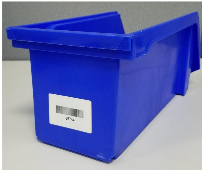
Figure 4. Bin with Radio Frequency Identification (RFID) tag
