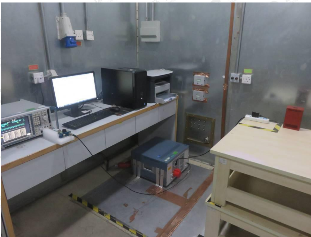
FCC RADIATED EMISSION TEST SETUP
