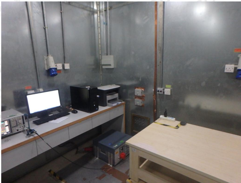
RADIATED EMISSION TEST SETUP
