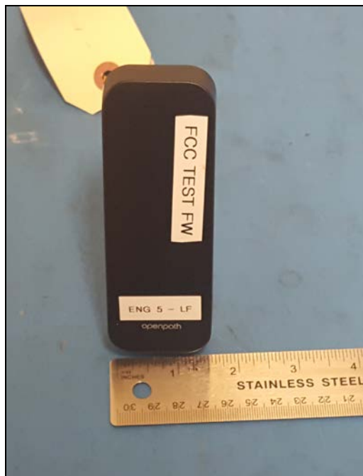
Photograph 1. Openpath Security Inc. Smart Reader & Mullion Smart Reader (LF) with Rigado BMD-340
