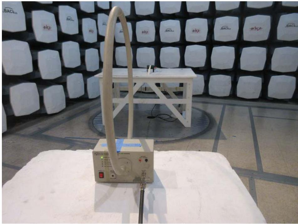
**1.4. 30 MHz – 1 GHz Loop: Perpendicular at 3 meters Rear View**
