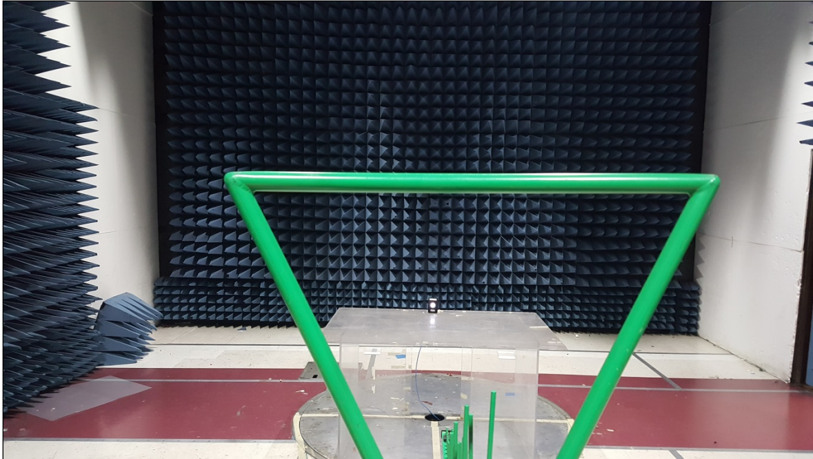
Photograph 3. Spurious Emissions, Test Setup, 30 MHz – 1 GHz
