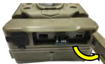
1. Open Controls Compartment Door. With Camera in 'OFF' Position Insert Micro SD Card into Micro SD Slot. A "click" sound indicates card is installed correctly.
