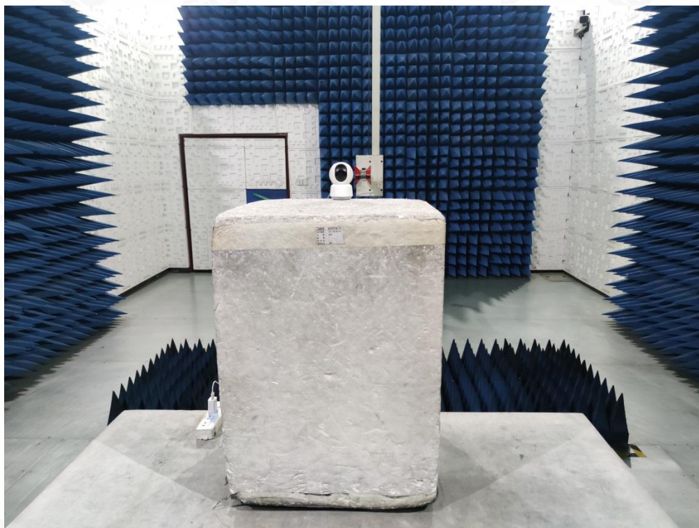
FCC RADIATED EMISSION TEST SETUP ABOVE 1GHZ
