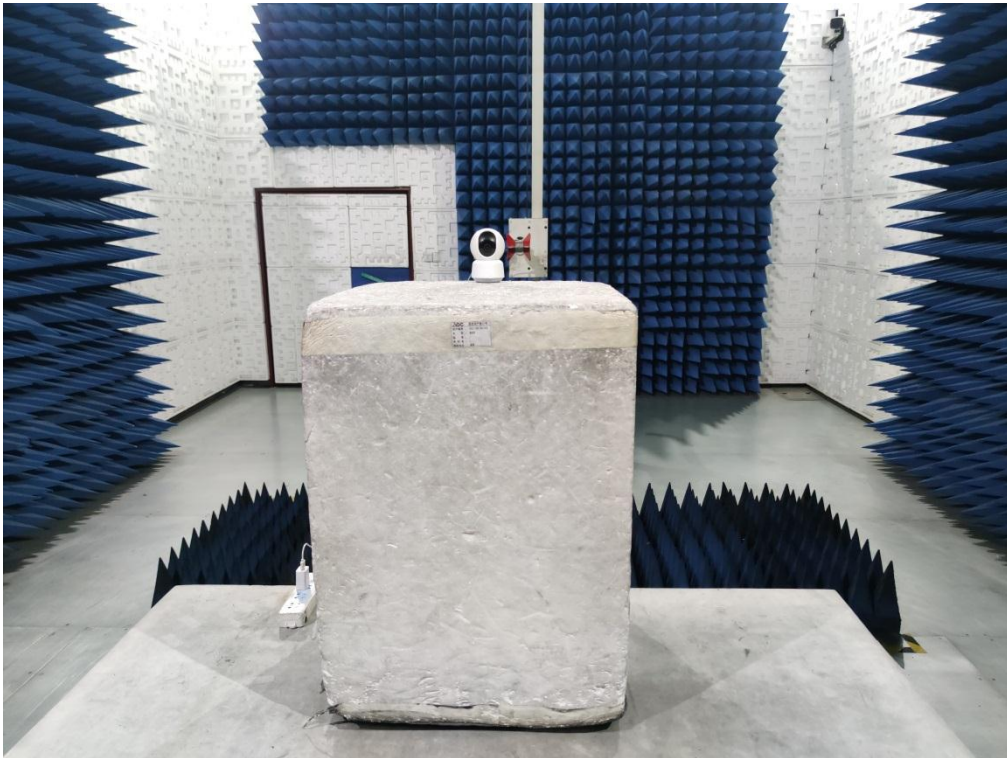
FCC RADIATED EMISSION TEST SETUP ABOVE 1GHZ
