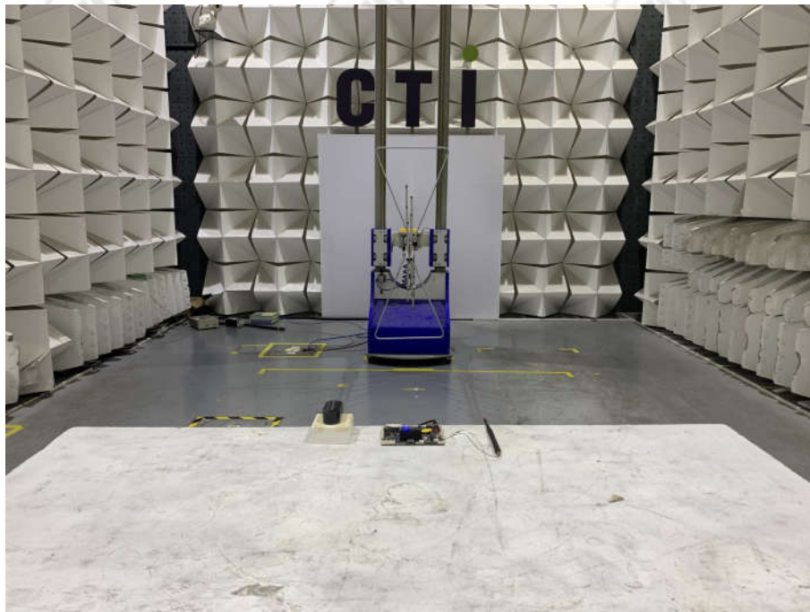
Radiated spurious emission Test Setup-1(Below 1GHz)
