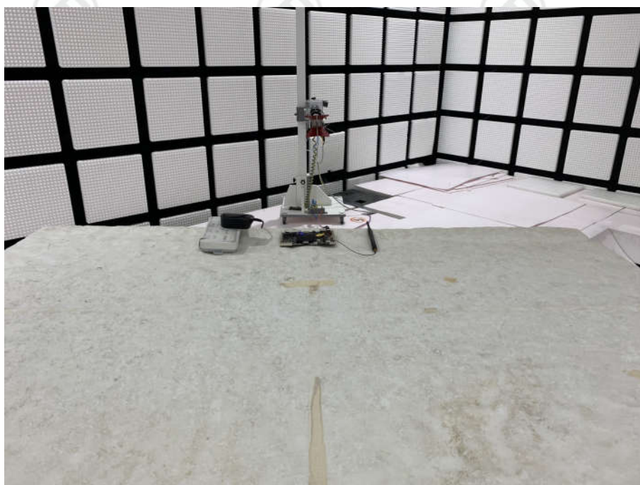
Radiated spurious emission Test Setup-2(Above 1GHz)
