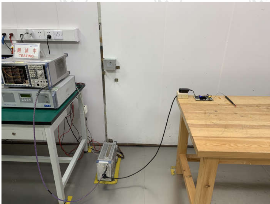
Conducted Emissions Test Setup
