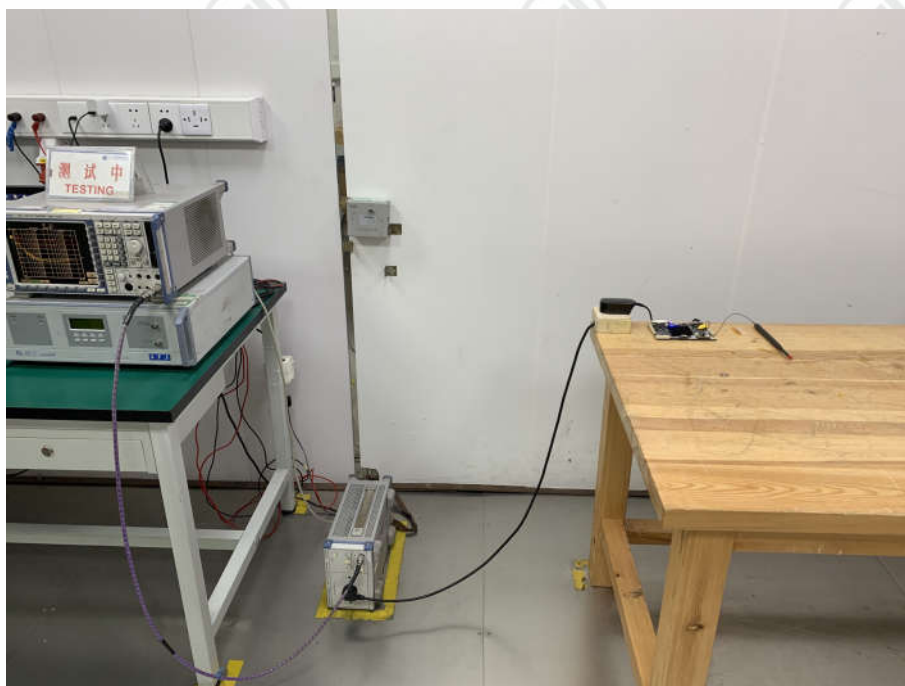
Conducted Emissions Test Setup
