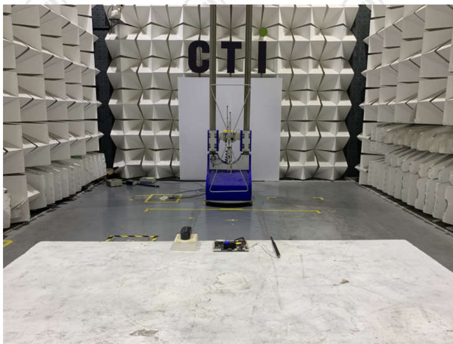
Radiated spurious emission Test Setup-1(Below 1GHz)
