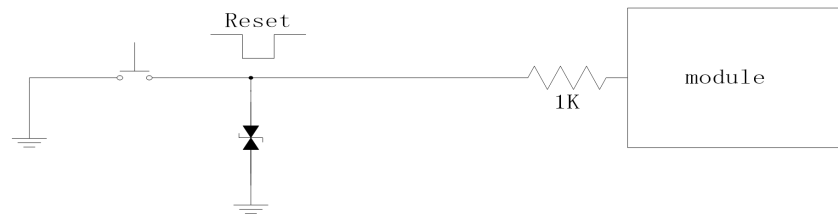
Figure 4.7: Reference design of key reset circuit
