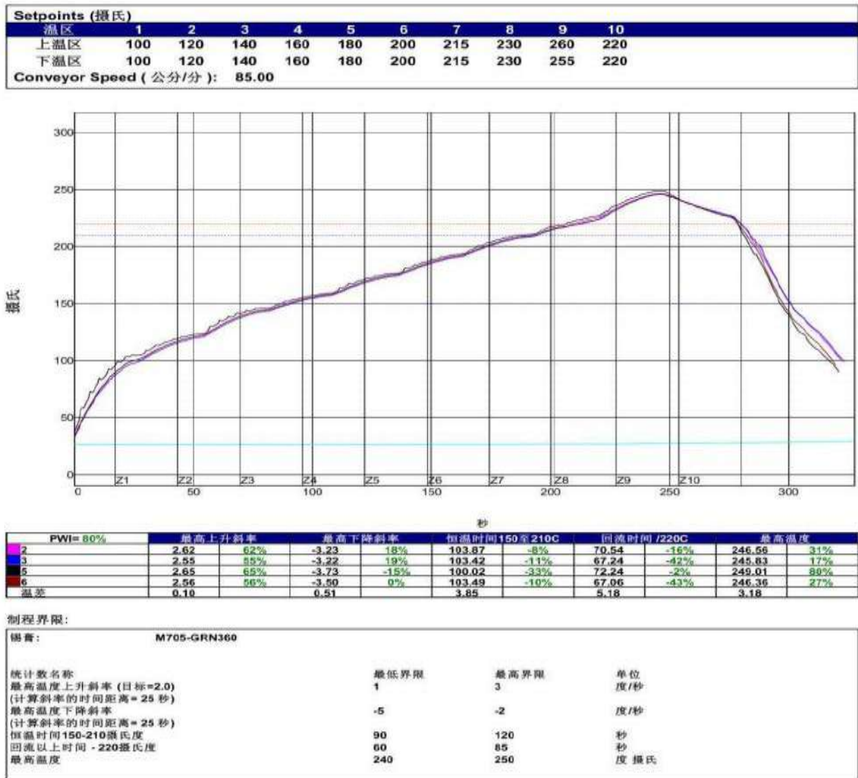
Figure 35 Reflow temperature curve
