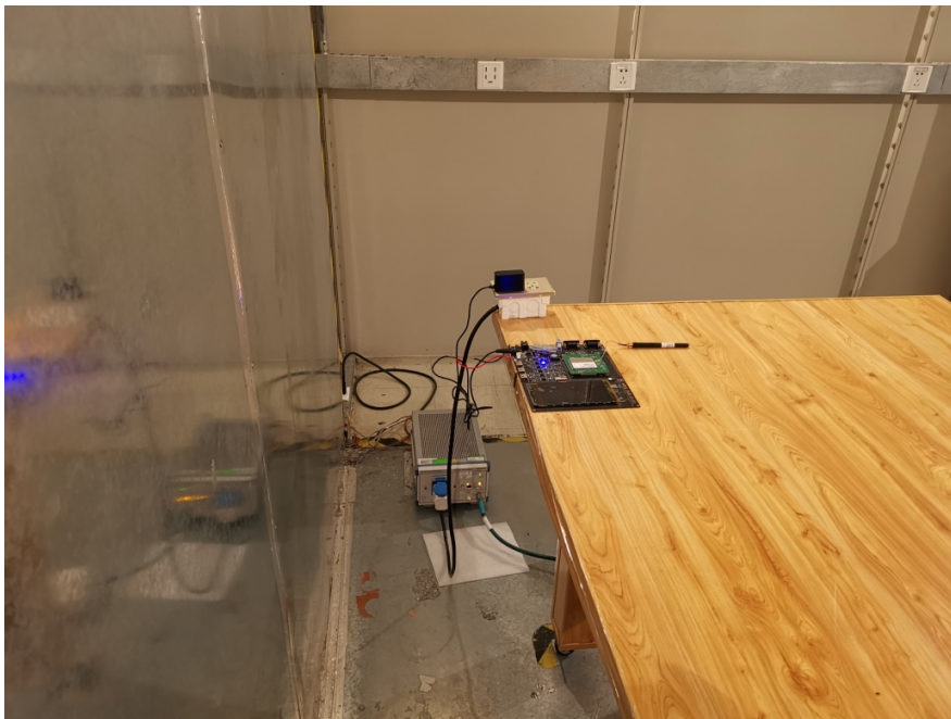
Conducted Emissions Side View
