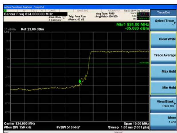
LTE Band 26 16QAM 15MHz CH-Low 100%RB
