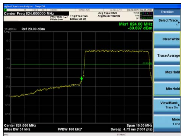
LTE Band 26 16QAM 10MHz CH-Low 1RB
