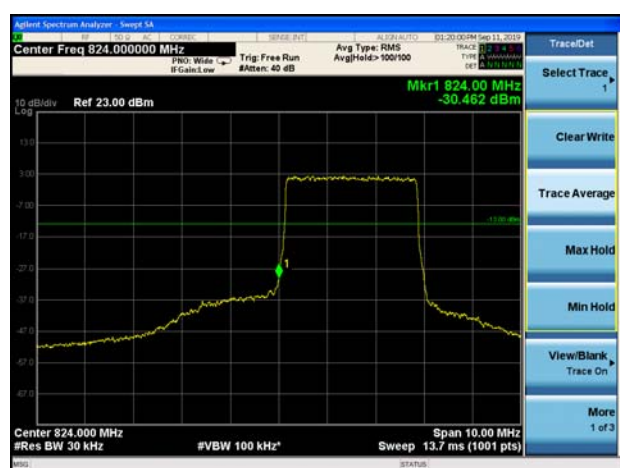
LTE Band 26 16QAM 5MHz CH-Low 1RB
