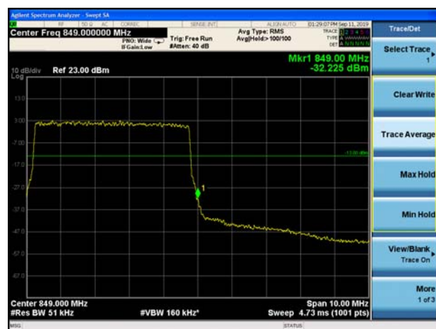
LTE Band 26 16QAM 10MHz CH-High 1RB
