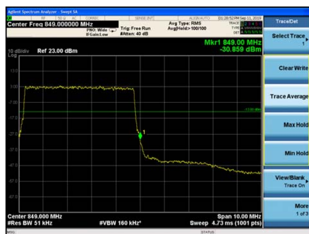
LTE Band 26 QPSK 5MHz CH-High 100%RB
