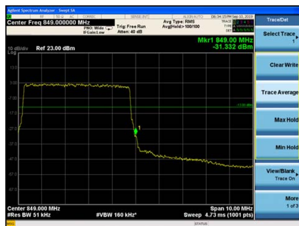
LTE Band 5 16QAM 10MHz CH-High 1RB
