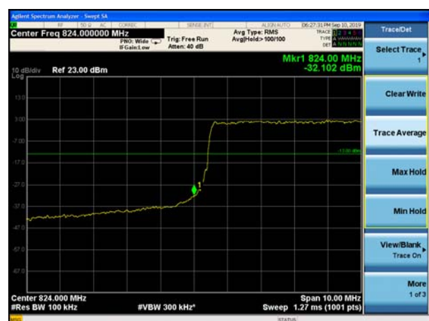
LTE Band 5 16QAM 10MHz CH-Low 100%RB
