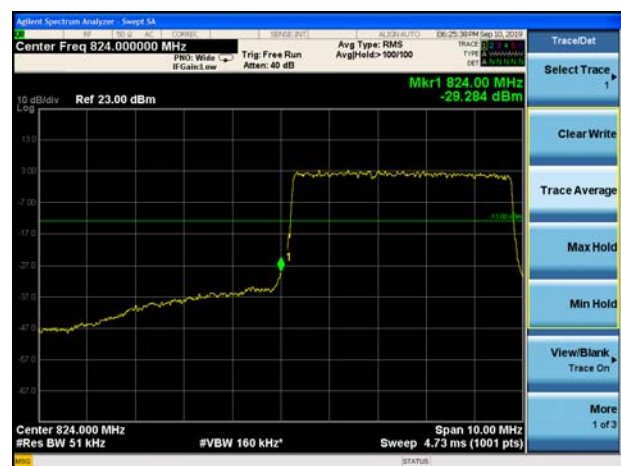
LTE Band 5 16QAM 10MHz CH-Low 1RB
