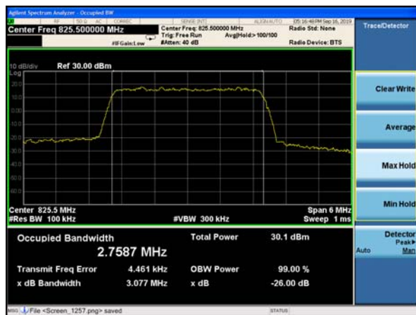
LTE Band 26 16QAM 3MHz CH-Middle
