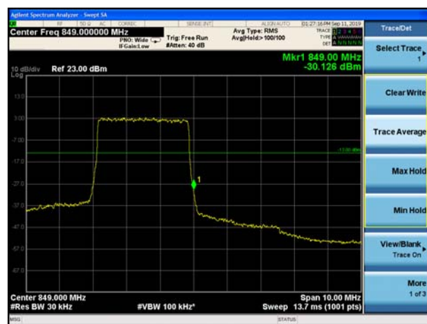
LTE Band 26 QPSK 5MHz CH-High 1RB
