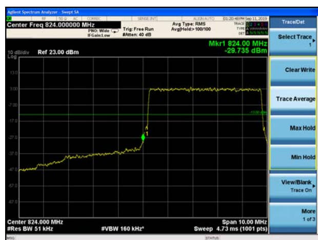
LTE Band 26 QPSK 5MHz CH-Low 100%RB
