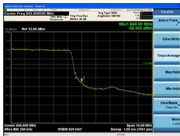
LTE Band 26 16QAM 1.4MHz CH-High 1RB
