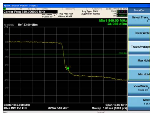
LTE Band 26 16QAM 10MHz CH-High 100%RB
