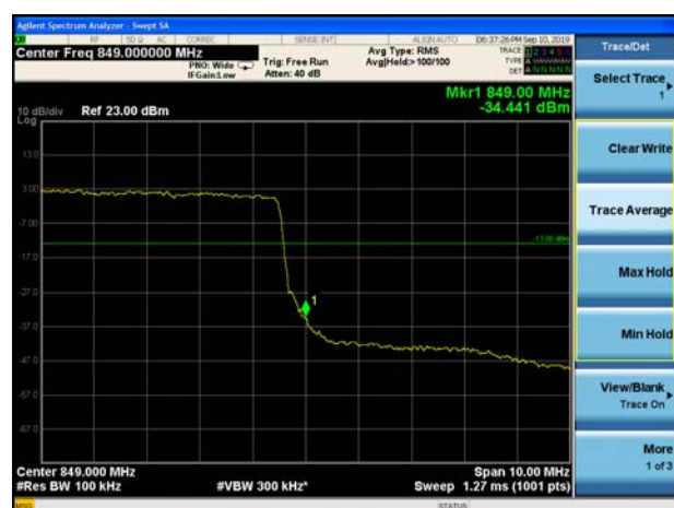
LTE Band 5 16QAM 10MHz CH-High 100%RB
