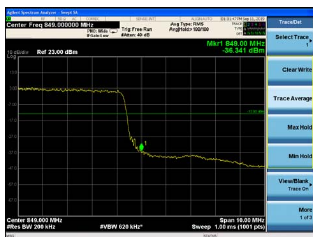
LTE Band 26 16QAM 15MHz CH-High 100%RB
