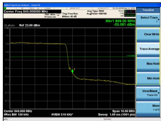
LTE Band 26 QPSK 15MHz CH-High 1RB
