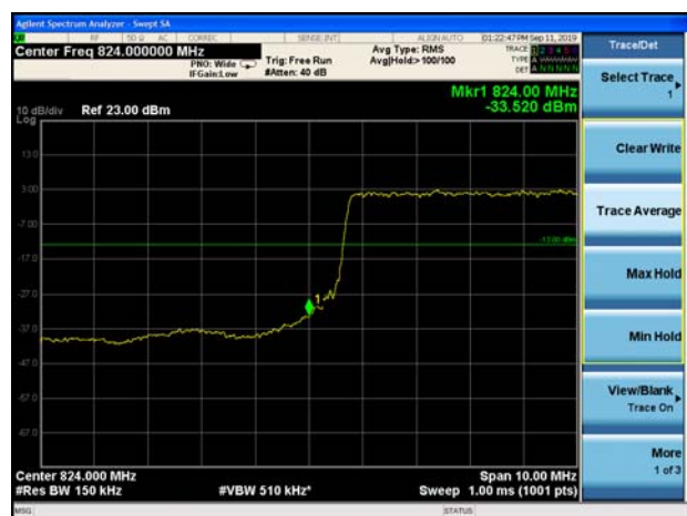
LTE Band 26 16QAM 1.4MHz CH-Low 1RB
