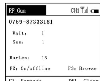
Wireless Barcode Collector still allows barcodes to be scanned and cached automatically in the event of occasional outages, for a maximum of about 1000 barcodes at a time. When the communication is restored, the PDT Series will automatically send the buffered barcode to the base station.
