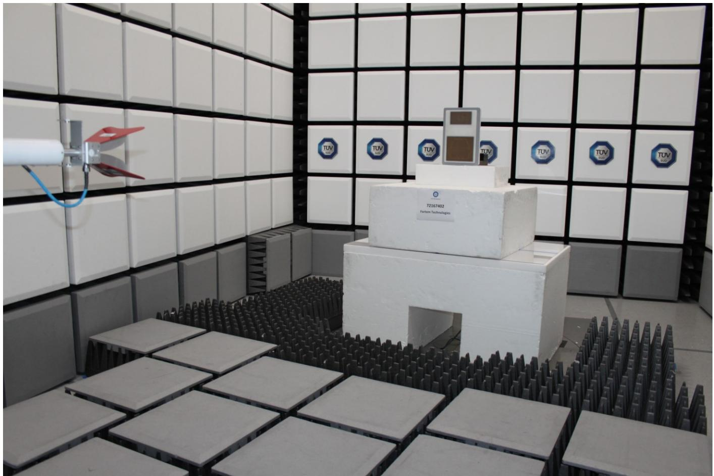
**Radiated Emissions Test Setup (1GHz to 40GHz)**
