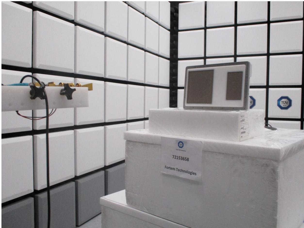
**Radiated Emissions Test Setup (above 40GHz)**
