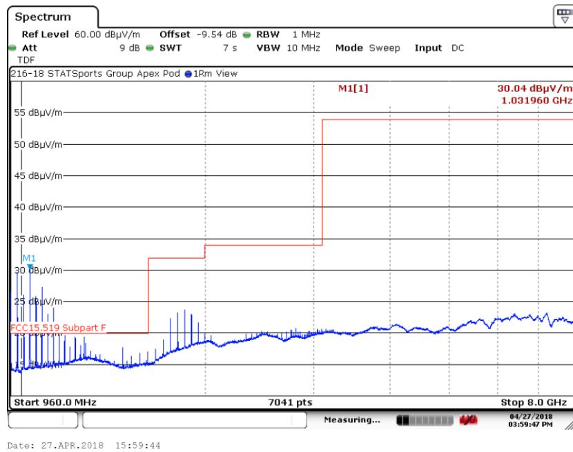
6.5.14. 960 MHz to 8 GHz Vertical at 1 Meter, -9.54 dB offset in analyzer No Tx
