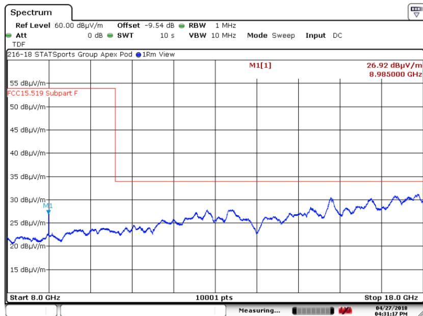
6.5.4. 8 to 18 GHz Vertical at 1 Meter, -9.54 dB offset in analyzer CH3 16M
