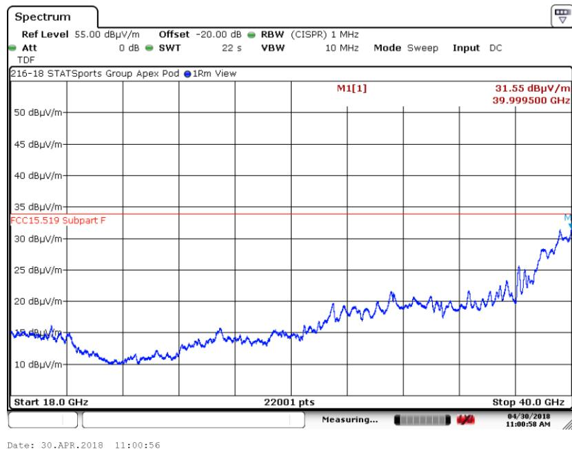
6.5.6. 18 to 40 GHz Vertical at 0.3 Meter, -20.00 dB offset in analyzer CH3 16M
