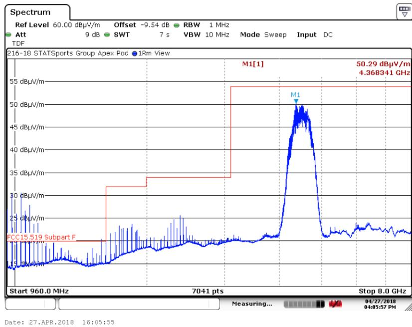
6.5.8. 960 MHz to 8 GHz Vertical at 1 Meter, -9.54 dB offset in analyzer CH3 64M
