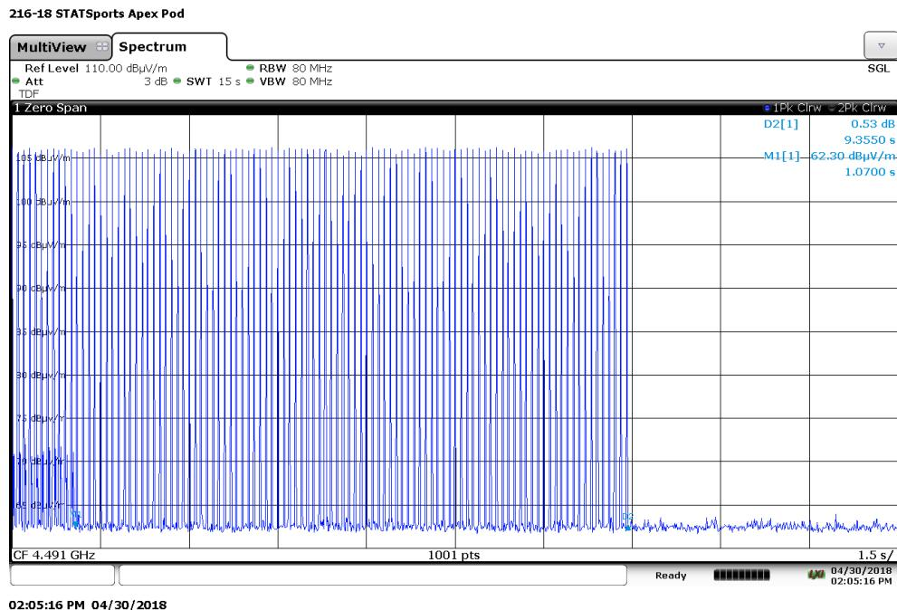
**Note:** Marker 1 is when the anchor (support equipment) stops transmitting, Marker D2 shows the EUT shutting off after 9.355 Seconds.
