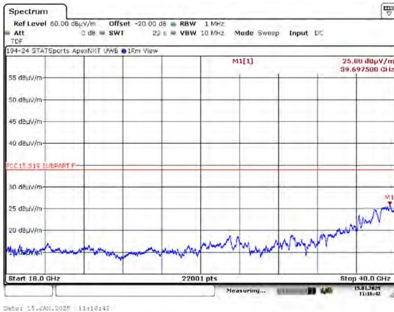
6.5.50. 18 to 40 GHz Vertical at 0.3 Meter – Channel 5, 16M, X-Axis
