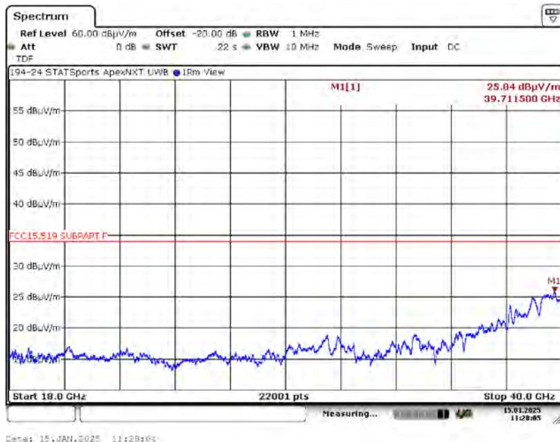
6.5.54. 18 to 40 GHz Vertical at 0.3 Meter – Channel 5, 16M, Z-Axis
