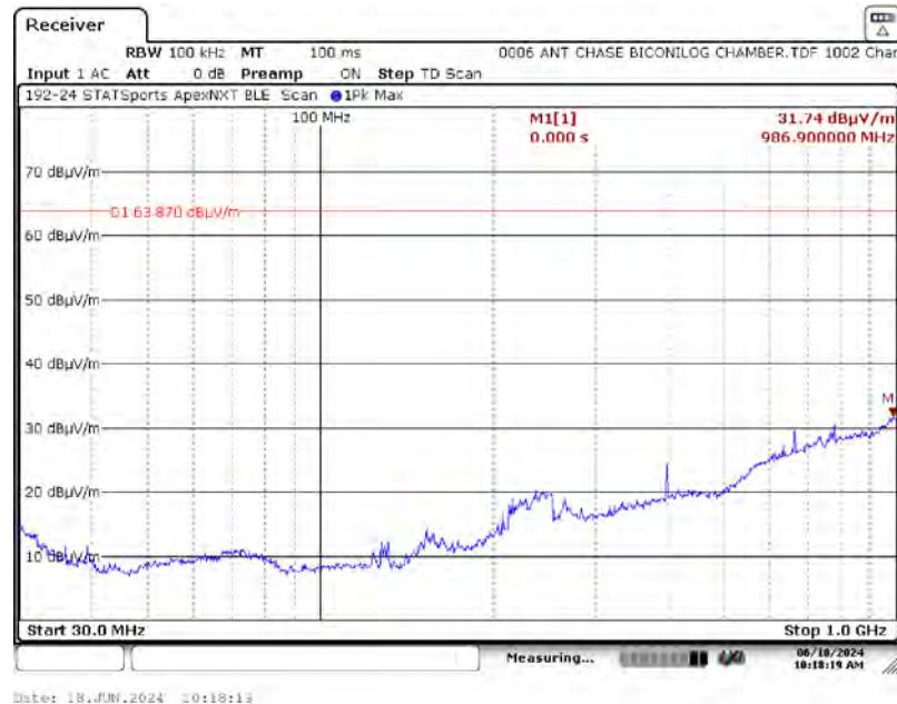
**B1.1.6. Measurement Results, 2480 MHz, 30 MHz – 1 GHz, Vertical, Z-Axis**
