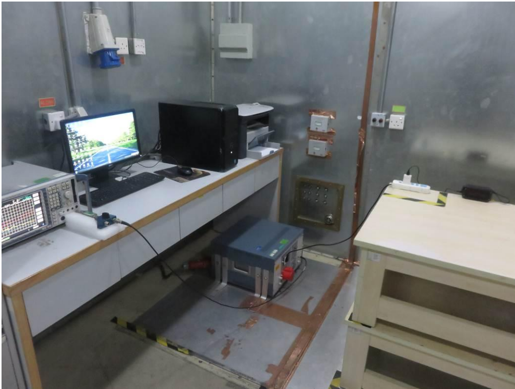
FCC RADIATED EMISSION TEST SETUP
