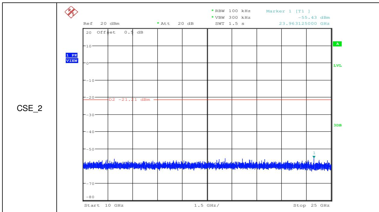
RF Conducted Spurious Emissions\_11N20SISO\_2437\_Ant1
