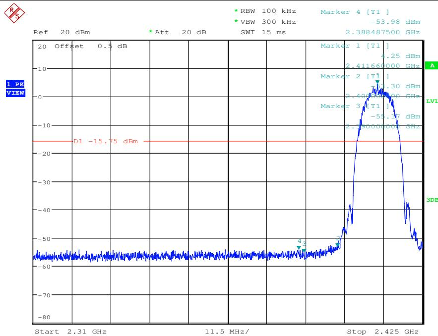
Band-edge for RF Conducted Emissions\_11B\_2462\_Ant1
