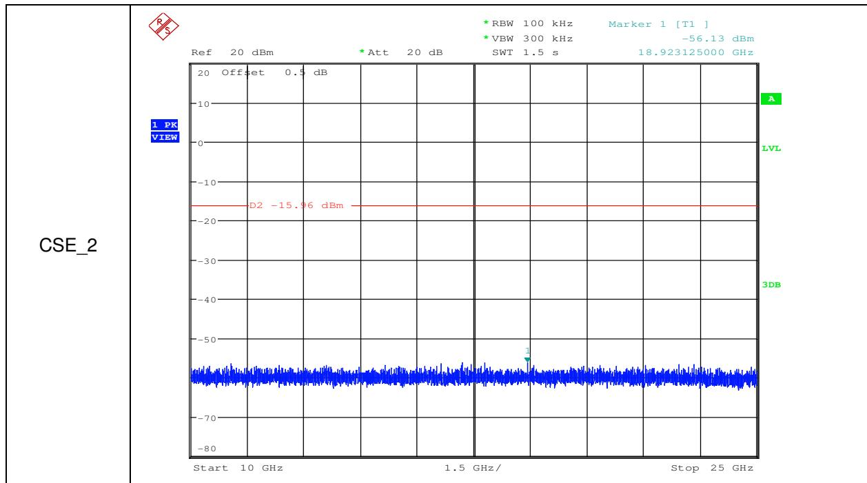
RF Conducted Spurious Emissions\_11B\_2437\_Ant1
