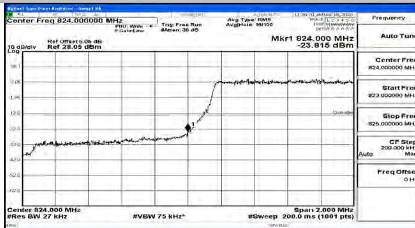
Band Edge Test Graph(s) (Channel Bandwidth: 1.4 MHz)_LCH_QPSK
