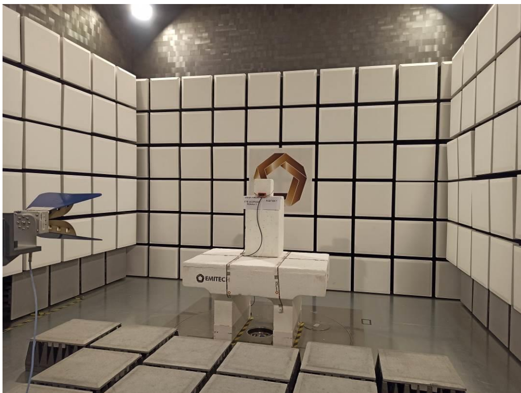
TEST SETUP PHOTO(S) - MAXIMUM PEAK OUTPUT POWER OF UWB DEVICE
