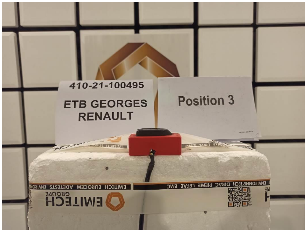
TEST SETUP PHOTO(S) - MAXIMUM PEAK OUTPUT POWER OF UWB DEVICE / POSITION 3
