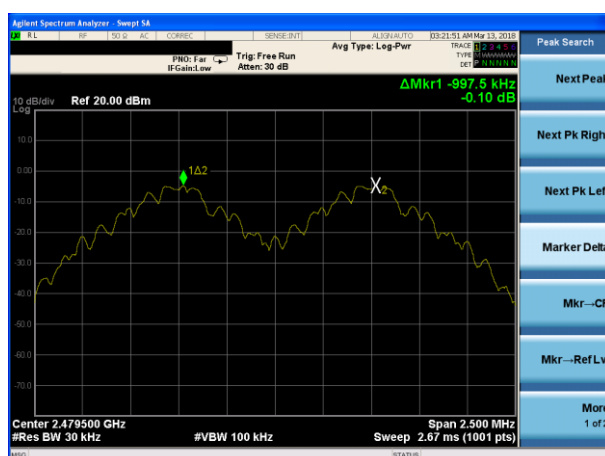
(1Mbps) Channel Separation plot on channel 77-78
