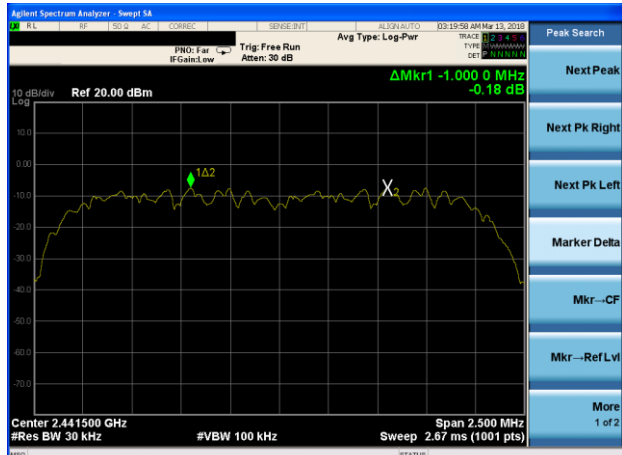
(2Mbps) Channel Separation plot on channel 39-40
