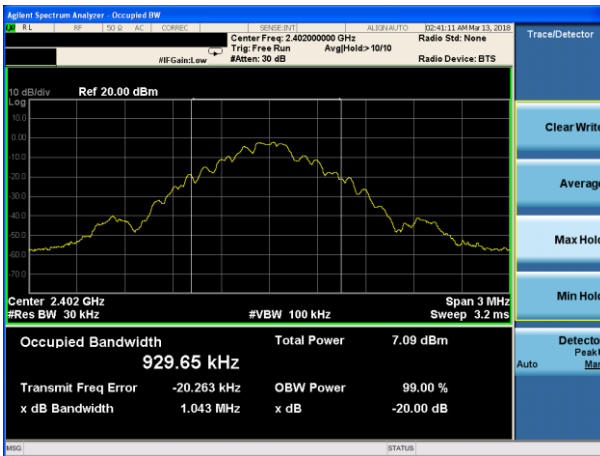
20dB Bandwidth plot on channel 39 (1Mbps)
