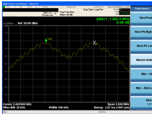
(1Mbps) Channel Separation plot on channel 39-40
