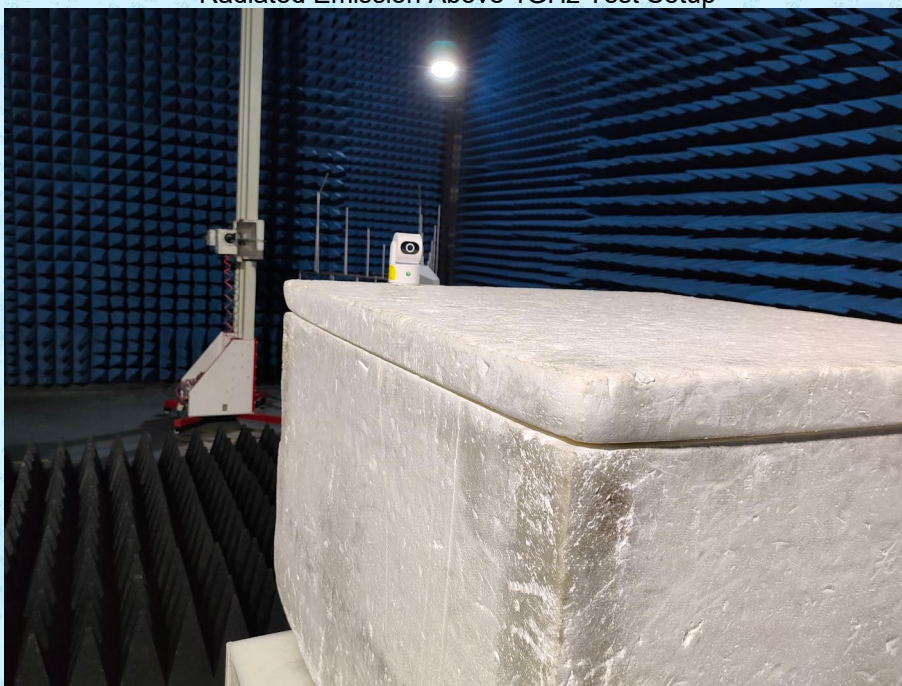
Radiated Emission Above 1GHz Test Setup
