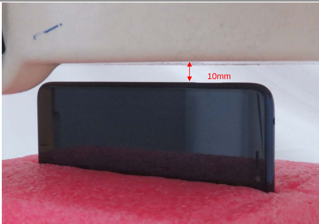
Picture 7: Left Side, the distance from handset to the bottom of the Phantom is 10mm
