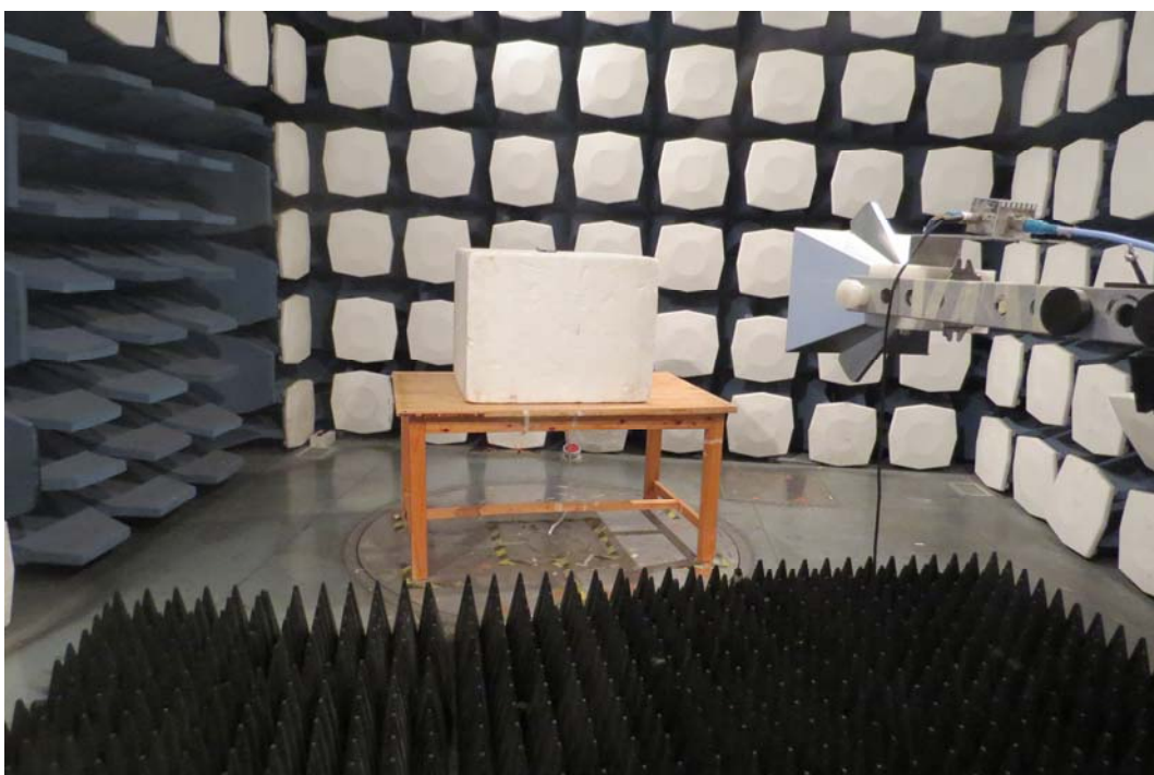
Picture 1: Radiated Spurious Emissions Test setup
