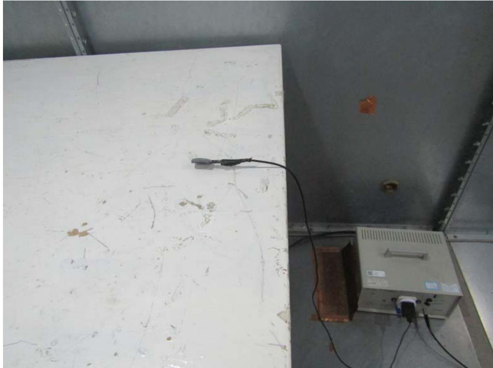
Measurement of Conducted Emission Test Set Up
