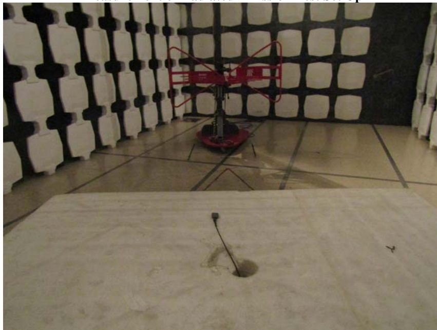
Measurement of Radiated Emission Test Set Up
