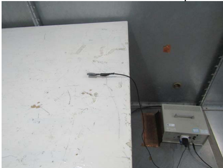
Measurement of Conducted Emission Test Set Up
