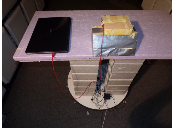
Radiated emission (Test setup for frequency <1GHz, pre-scan)
