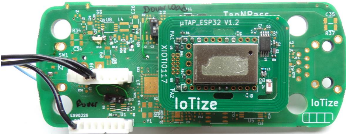
Tested Sample mounted on a expansion board
