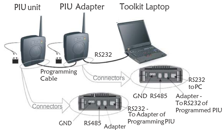
Figure 23 PIU Adapter Programming Mode Connections
