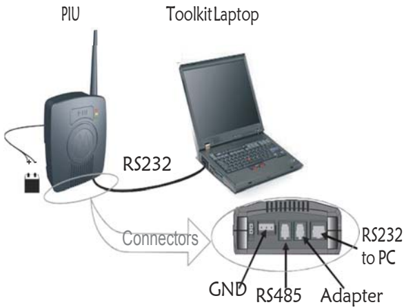
Figure 22 PIU Adapter – PC Communication Connections
