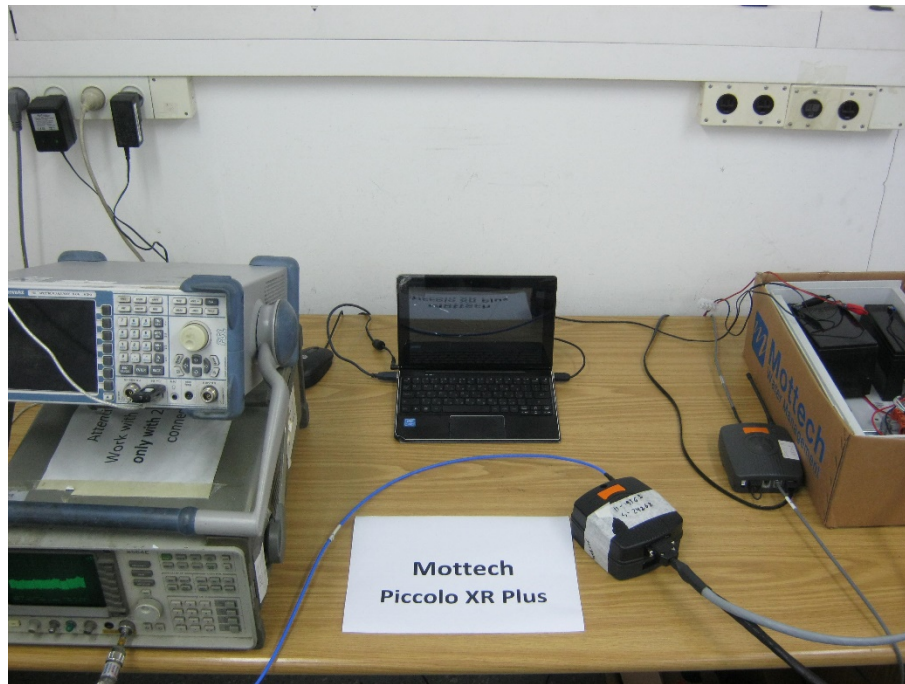
Figure 3. Conducted Emission from Antenna Ports Test
