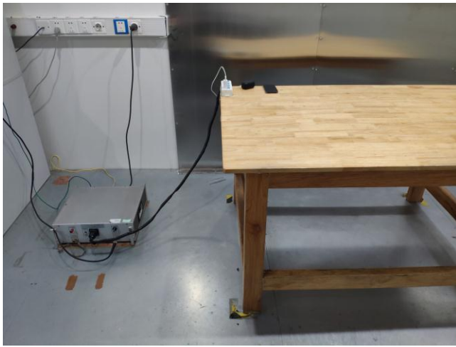
Conducted Emissions Test Setup Front View
