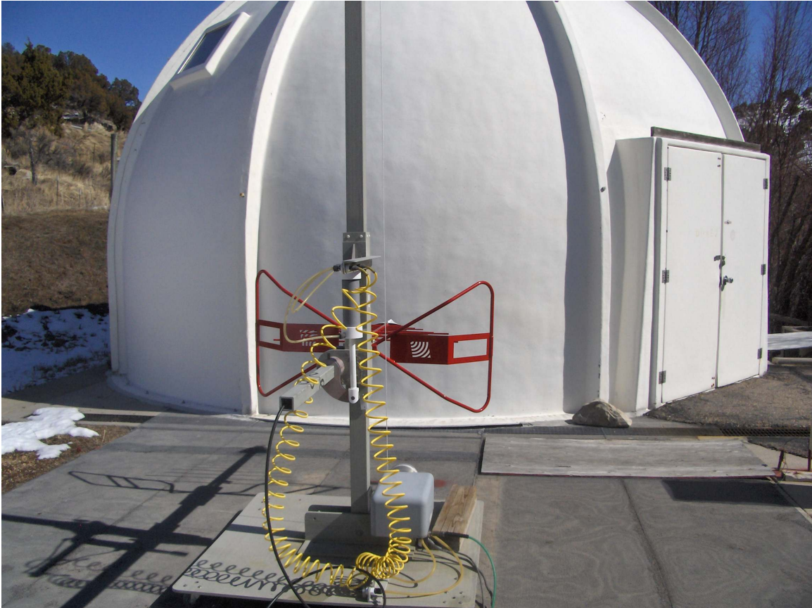
Test Set Up - Radiated Emissions 30MHz to 1000MHz - Photo 05
