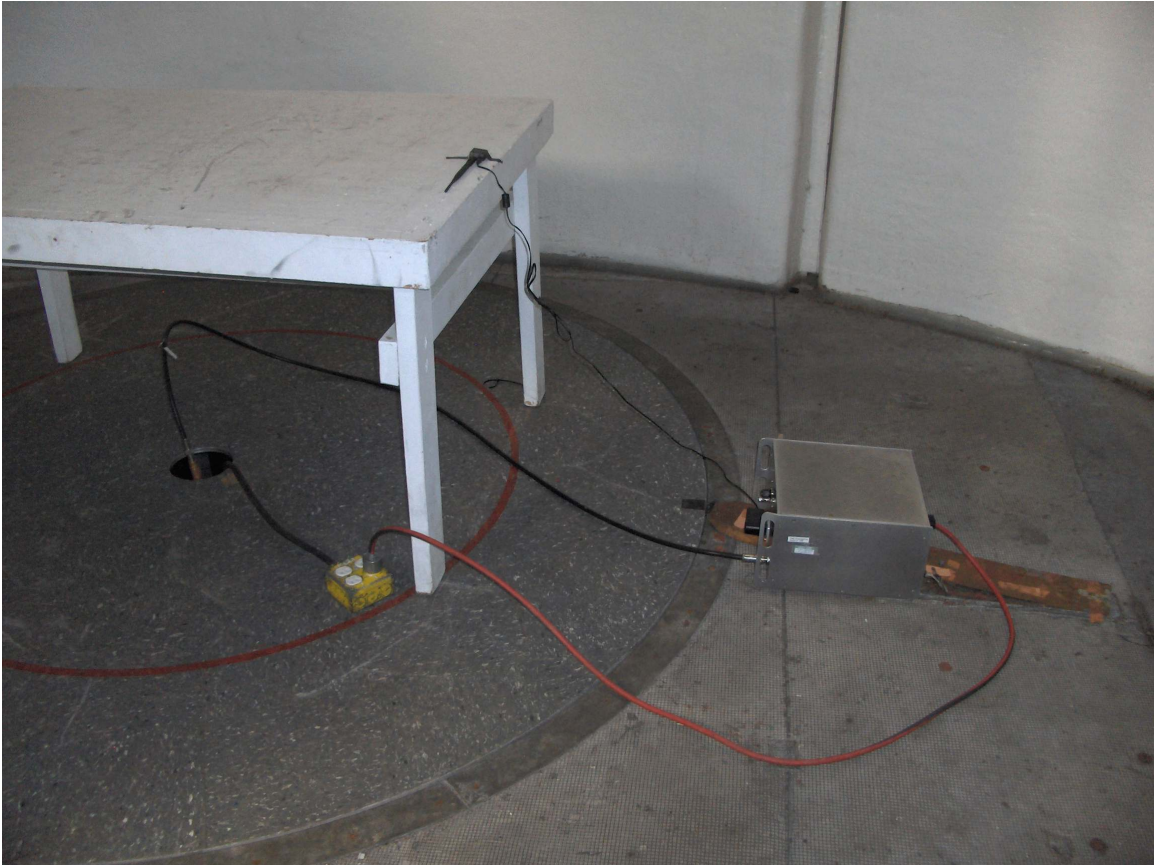
Test Set Up - Conducted Emissions with ferrite - Photo 01
