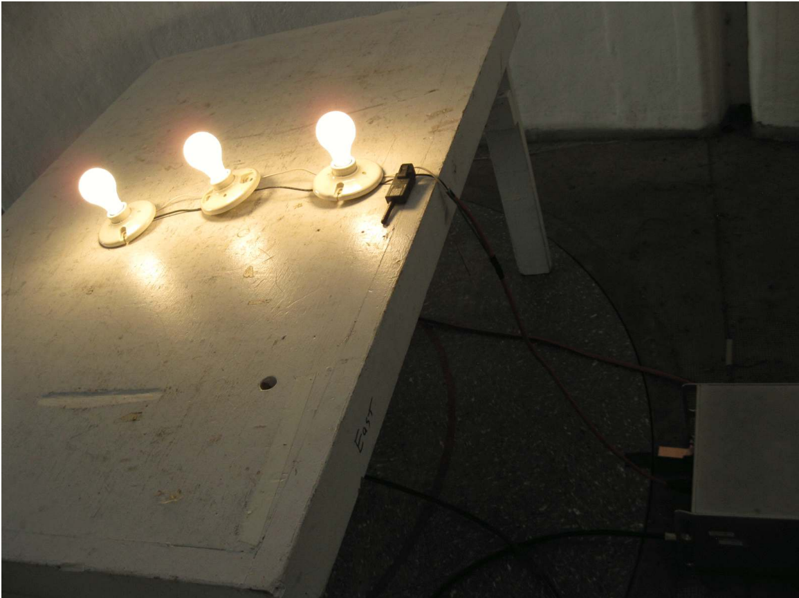
Test Set Up - Conducted Emissions - Energy Harvesting Method - Photo 11
