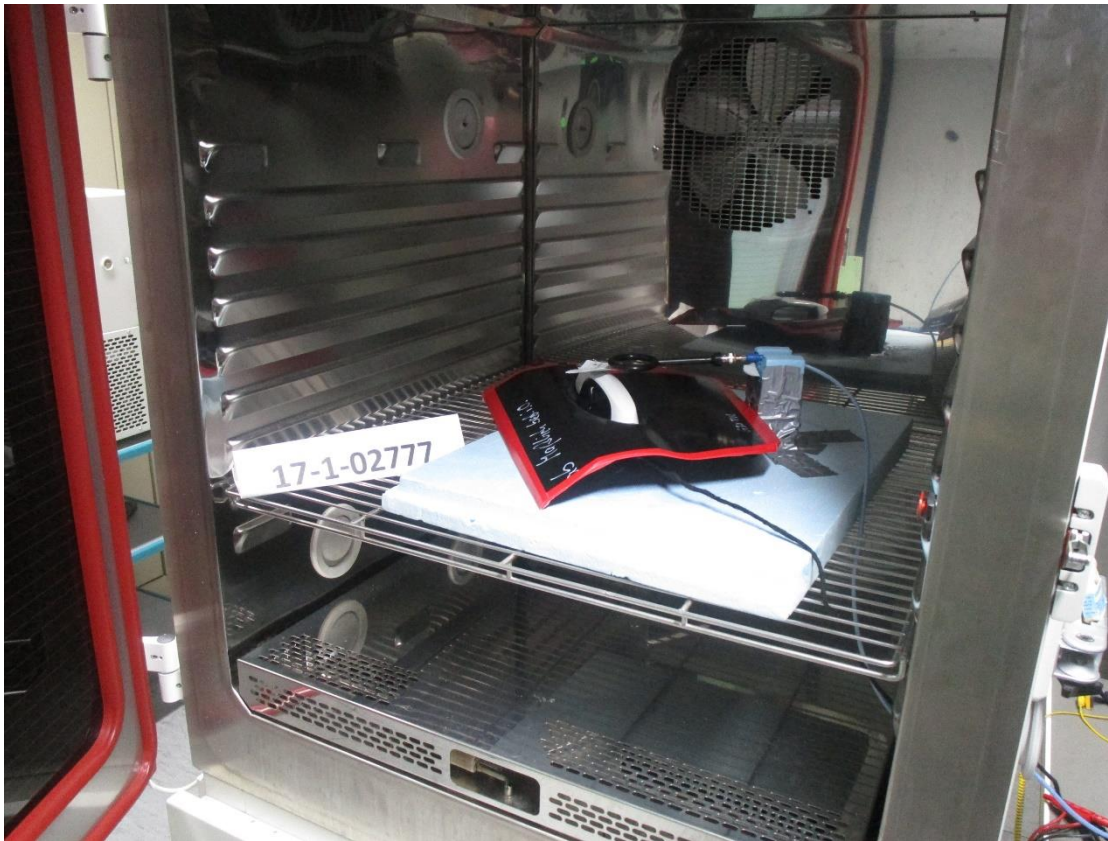
Diagram 7: Setup for radiated measurement in the radio laboratory, in the climate cabinet under extreme conditions (close view)
