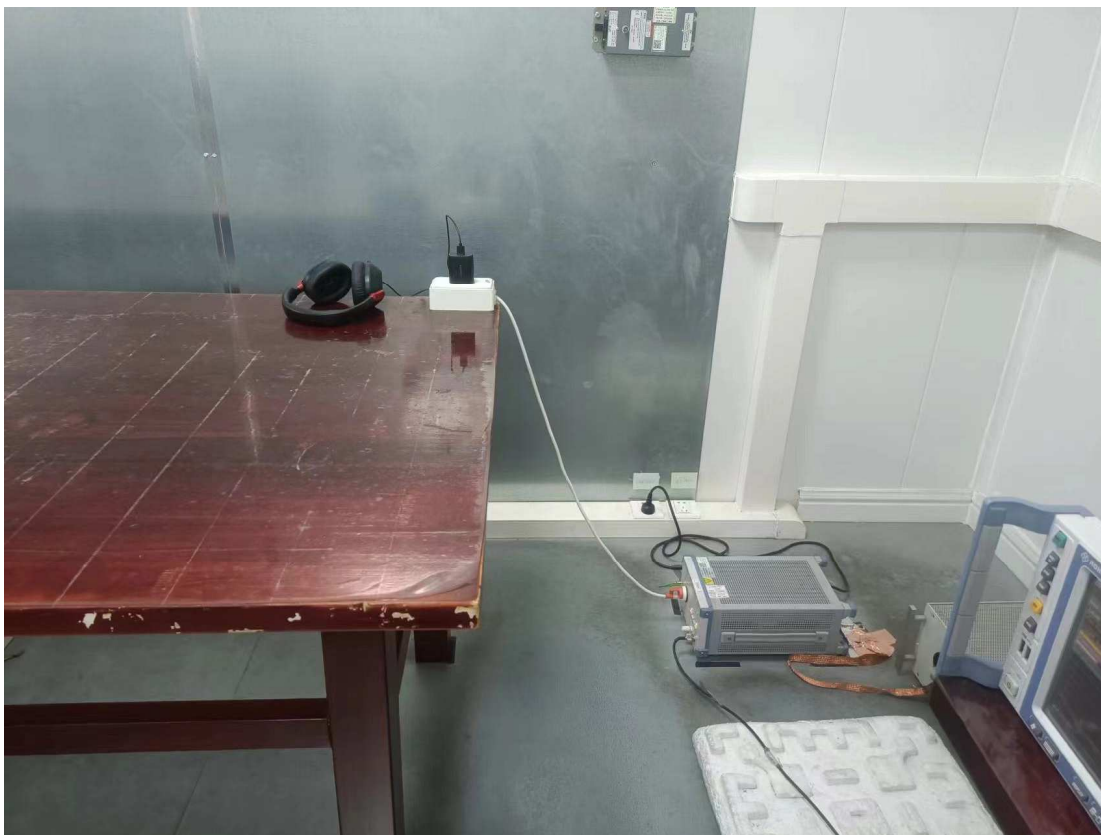
Photograph 3: Set-up photo for Conducted Emission
