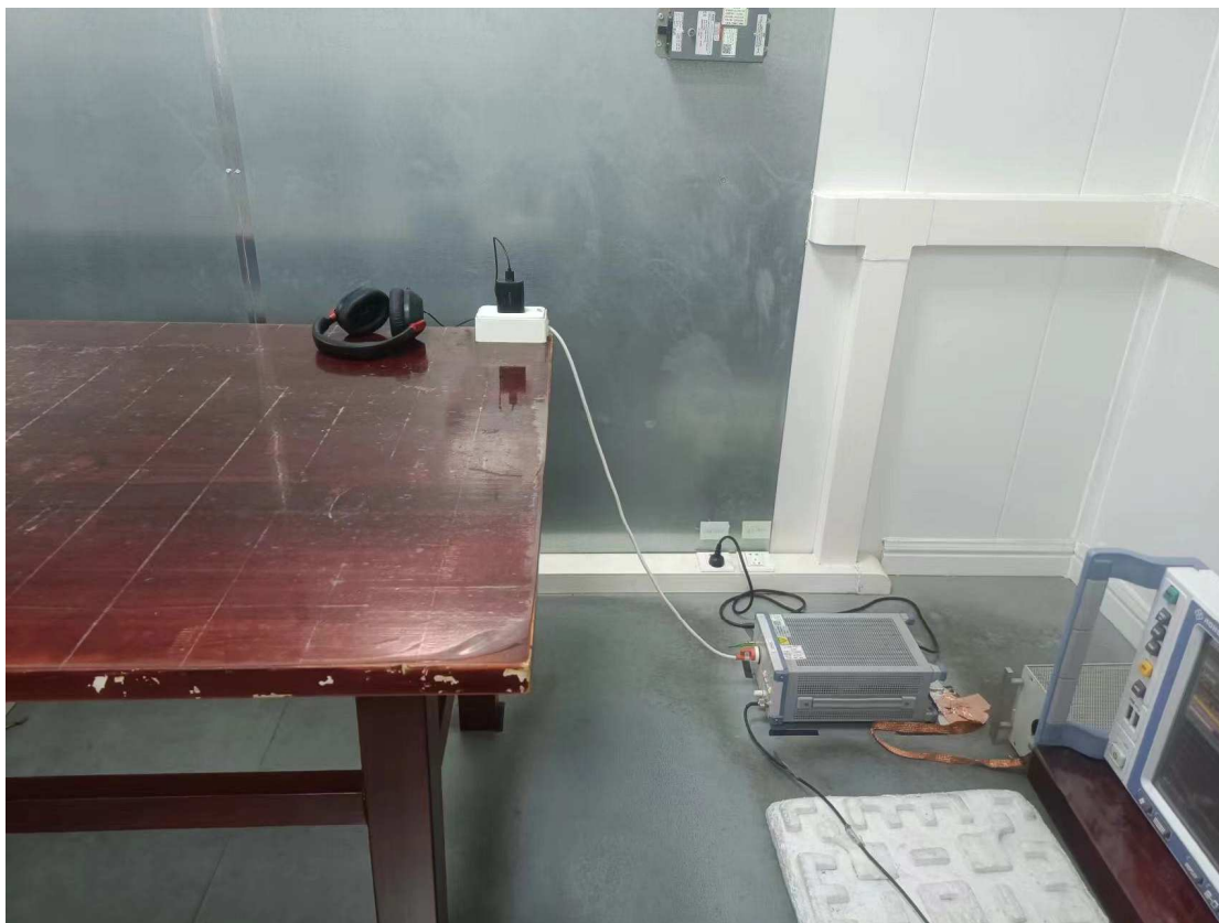
Photograph 3: Set-up photo for Conducted Emission
