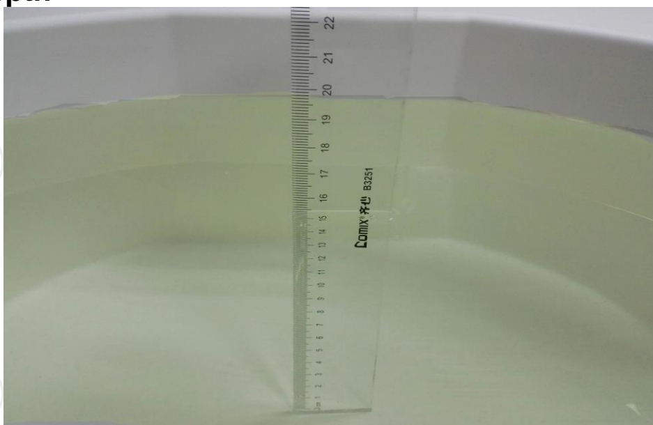
The Body Liquid of 835MHz (15.4cm)
